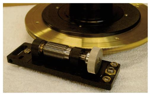
Image 1 - A high-precision stainless-steel worm screw (foreground) and bronze worm wheel (background) by Mathis Instruments machined to an accuracy of  $\pm 0.0001$  inches in residual run-out and thread lead error for native tracking accuracy of ~5.0-arc seconds peak-to-peak error.
