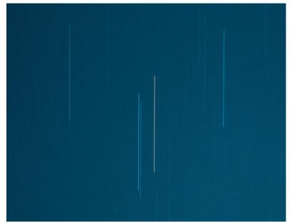
Image 11 - TA single 3.5-minute exposure at 300-mm, cropped to show detail, captured with the Lightrack II purposely misaligned by 60 degrees to show tracking error. Resolution of the imaging system was 2.95 arc seconds per pixel, so the images demonstrate absolutely minimal error.
